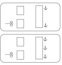
Attach the tether strap only to the appropriate tether anchor as shown. The tether strap may not work properly if attached somewhere other than the correct tether anchor.
